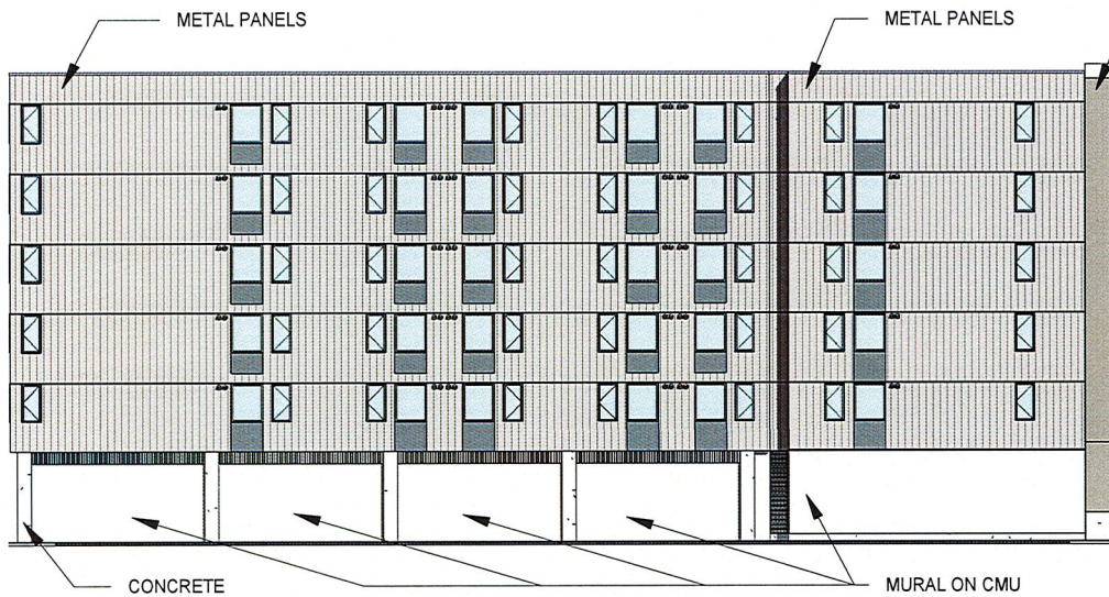
NORTH ELEVATION Alley
